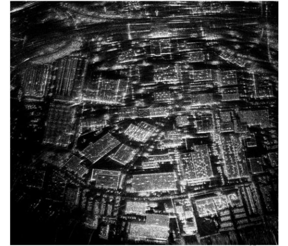
L-band SAR image: 200MHz bandwidth, res. < 1m
