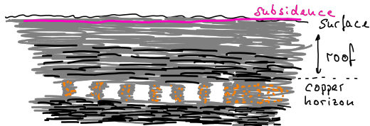
room-and-pillar mining scheme
