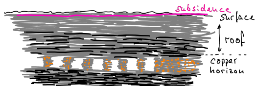
room-and-pillar mining scheme
